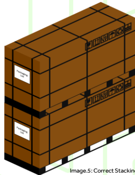
Image.5: Correct Stacking Layers of Modules.
